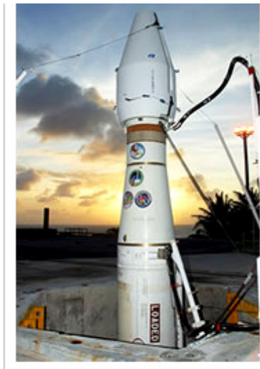
Raytheon's Exoatmospheric Kill Vehicle is the intercept component of the Ground Based Interceptor (GBI).
